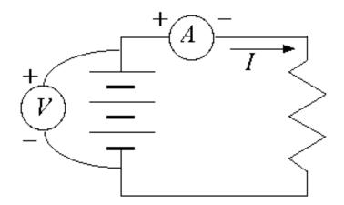
For the resistor in this circuit (if temperature is ~ constant), current is proportional to the potential difference across the resistor.
