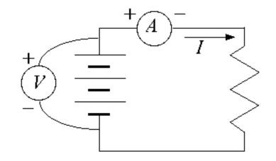
The proportionality factor *R* is the <u>resistance</u>. The unit for resistance is the ohm ( $\Omega$ ).
