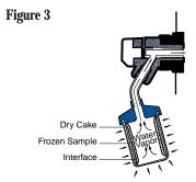
Ambient room temperature provides heat to encourage removal of water vapor from frozen samples when manifold drying.
