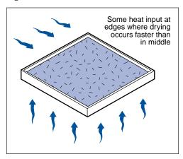
In bulk drying, heat is provided primarily through conduction from shelf.
