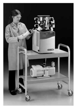
In the manifold drying method, flasks are individually attached to the ports of a drying chamber.
