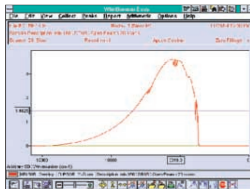
System response with the DTGS detector and quartz halogen source.
