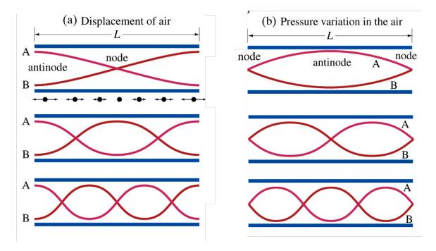
Again, note in the figure on the left above that even though the curves look identical to the transverse vibrations of a string, the vibrations of the particles are parallel to the direction of motion. To reinforce this concept, the displacement directions (and magnitudes) are displayed below the fundamental mode of the tube on the left.
