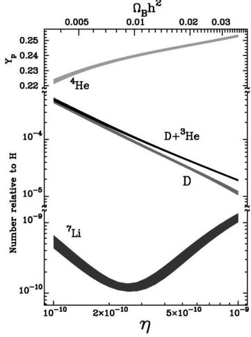
In the figure above, the helium fraction is denoted by  $Y_p$  (see the top left);  $Y_p$  is used to designate the primordial helium fraction of the Universe (that is, the helium fraction before nucleosynthesis begins in stars), and is a dimensionless number:
