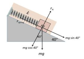
If we now consider the x-axis parallel to the incline and positive to the right, then the net force on the block:
